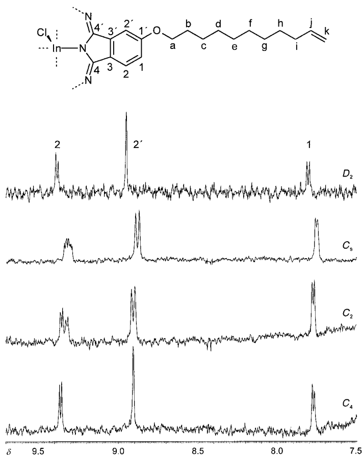
Figure 4. ^1\text{H} NMR spectra (600 MHz, 300 K) of the aromatic region of the separated pure isomers 1a–d measured by stopped-flow NMR spectroscopy.
